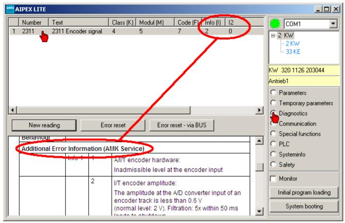
With 'Diagnostics', the diagnostic messages can be read out from the selected device.
