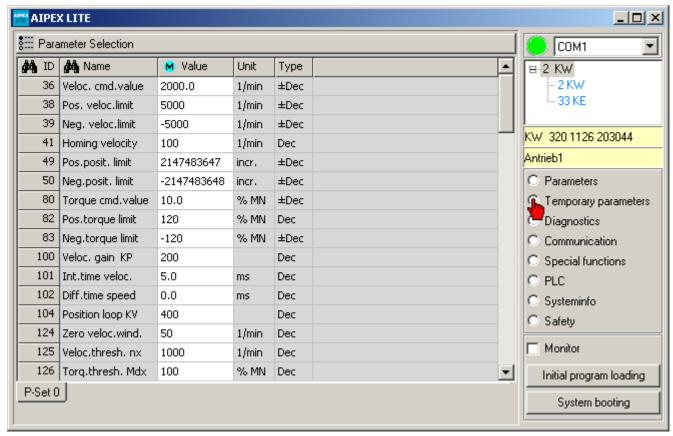
Changes in the 'Temporary parameters' are effective immediately in the drive. In the selection list, only parameters are offered that can be modified temporarily. All modified values are displayed in green font.
