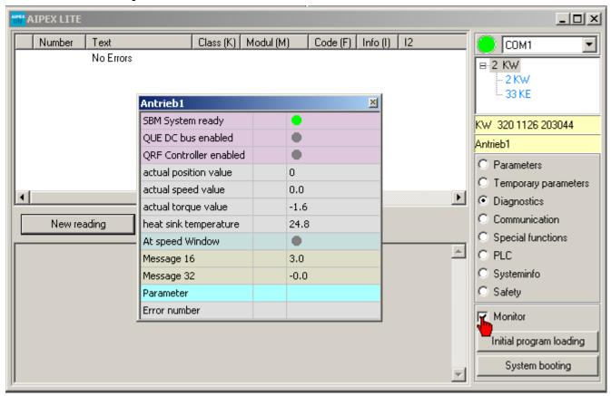
The 'Monitor' is a dynamic display of device data and statuses. A cyclic, but temporally undefined display of the values follows.
