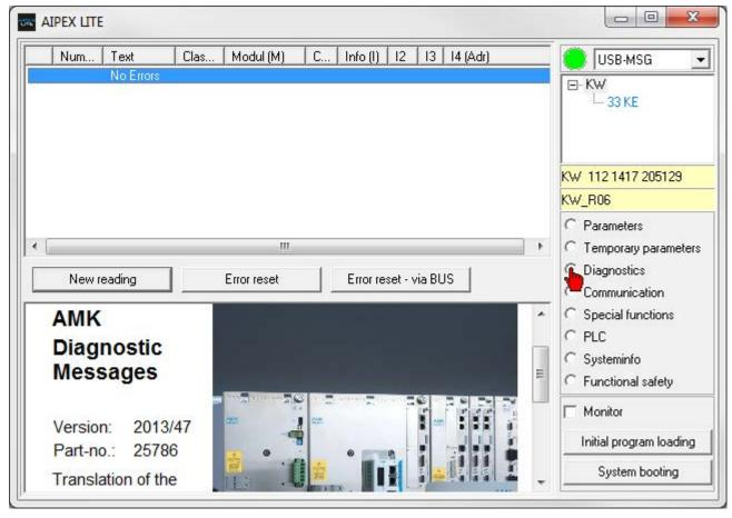
With 'Diagnostics', the diagnostic messages can be read out from the selected device.
