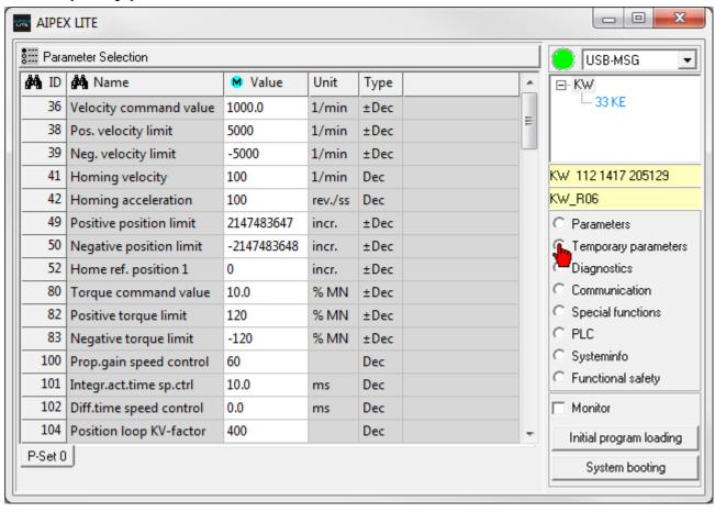
Changes in the 'Temporary parameters' are effective immediately in the drive. In the selection list, only parameters are offered that can be modified temporarily. All modified values are displayed in green font.
