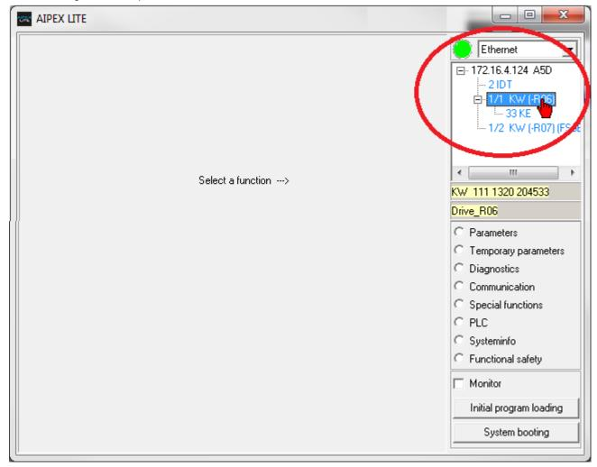
All active interfaces (connections between PC and AMK devices) are offered for selection.
