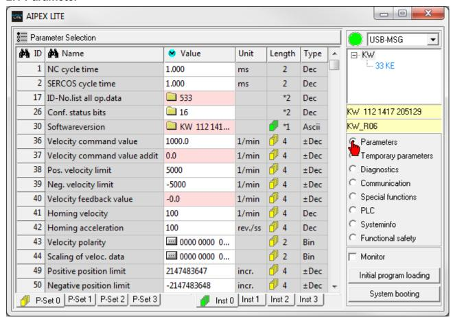
'Parameter' displays available offline and online values of the device selected in the device tree.
