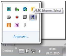
All active and manually created AMK Ethernet devices are displayed that were created in the title bar **device**. Select the device with which you want to establish a connection.
