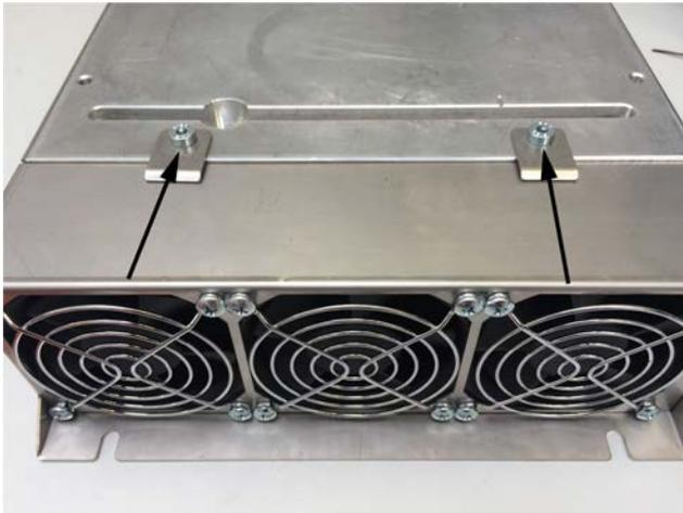
Mount holding clamps with cylinder screws M6 x 10
