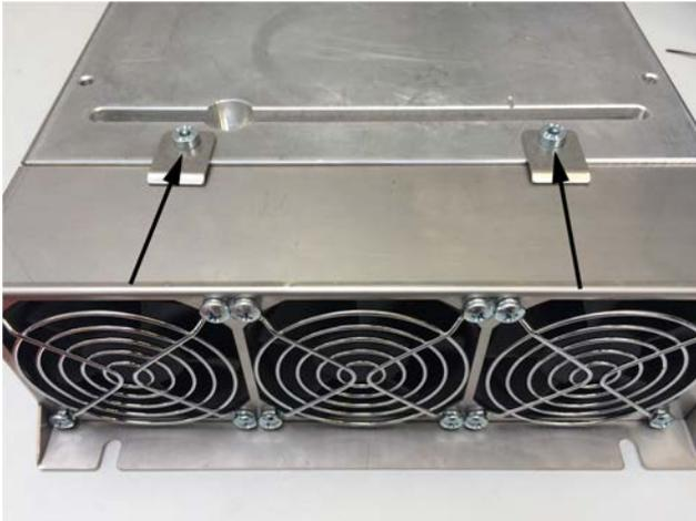
Remove holding clamps with cylinder screws M6 x 10
