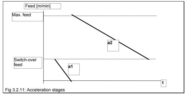
In the case of a contour interpolation the contour is limited with the acceleration of the slowest axis participating in the contour (also coupled axes). If a contour or coupled axis alone is moved, then its set acceleration stages apply for it.
