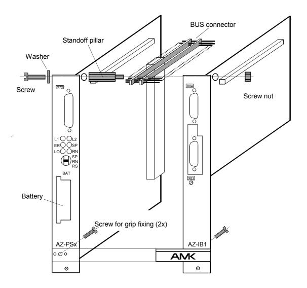
Assembly of AZ-PS5 and AZ-IB1 to AZ-PS5-I module (principle)
