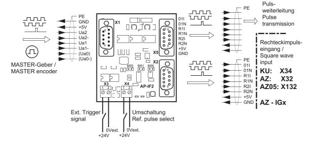
AP - IF2 Anschlüsse für Sinussignale / AP - IF2 connections for sine wave signals
