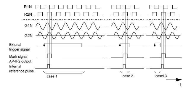
The external trigger signal or the encoder reference pulse can be output as the reference signal alternatively, selected via 24V binary input "Change-over":
