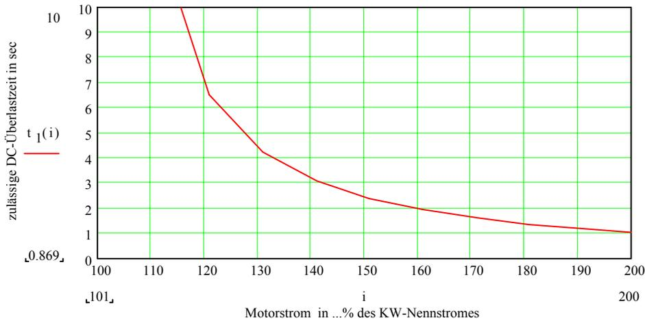
Motorstrom in ...% des KW-Nennstromes = Motor current in xx% of the KW current rating
