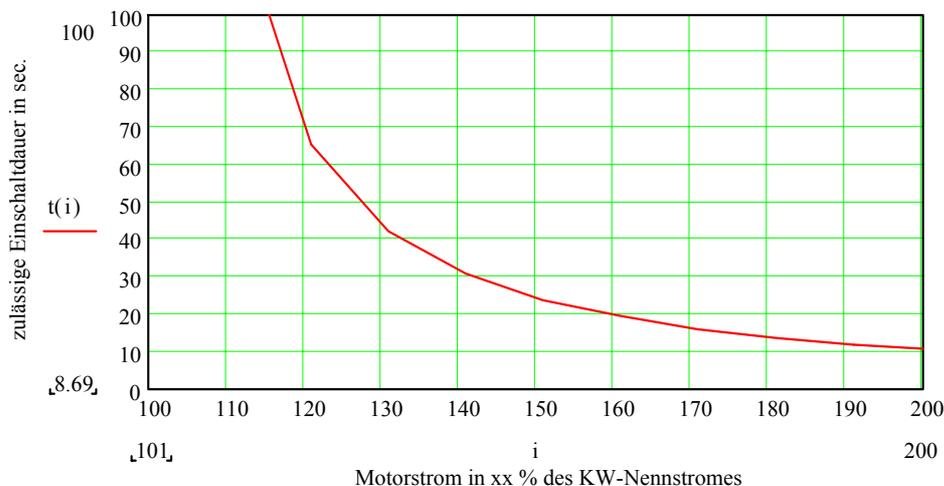
Motorstrom in xx% des KW-Nennstromes = Motor current in xx% of the KW current rating
