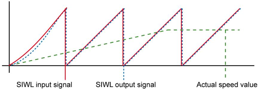
**Measurement 2:** ID34257 'SIWL control' Bit 6 = 1: Very fast control performance, without overshoot (monitor with 2 poles)
