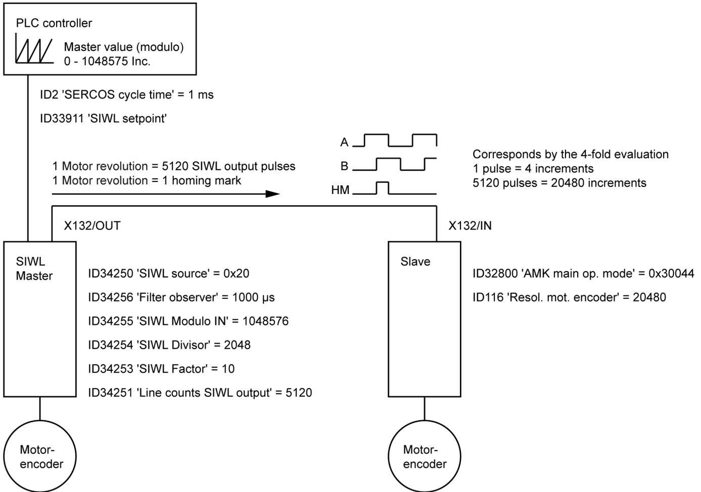
$$\text{SIWL output pulses per motor revolution} = \frac{\text{ID34255 'SIWL Modulo IN'}}{\text{ID34254 'SIWL Divisor'}} \times \text{ID34253 'SIWL Factor'}$$
