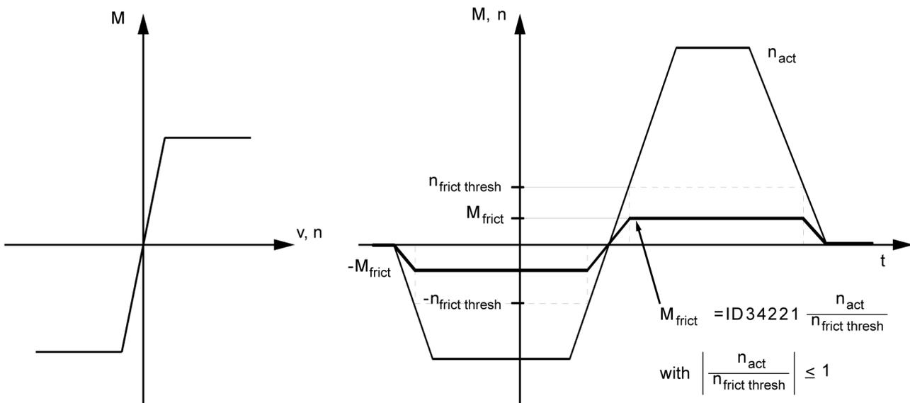
**ID34222 'Friction torque linear'**
