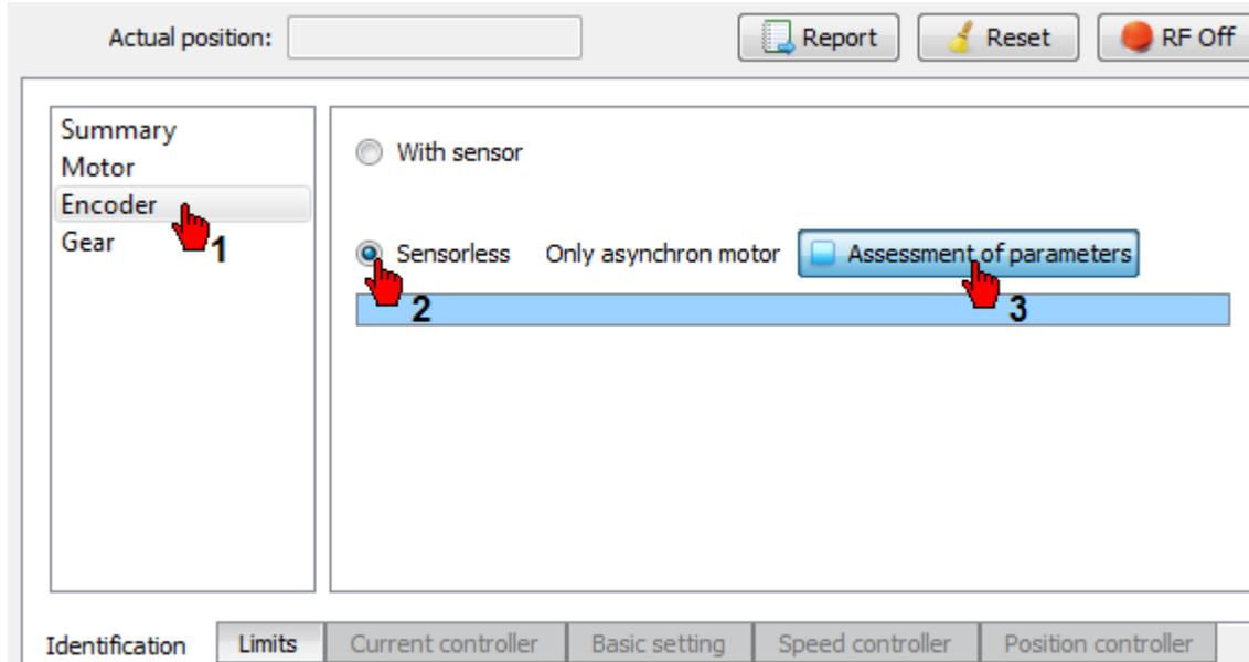
The 'Current Controller', 'Basic Settings', 'Speed Controller', and 'Position Controller' are not available when the 'Sensorless' function is selected.
