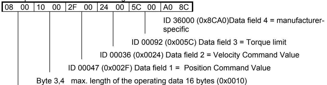
Byte 1,2 Length of the programmed operating data 8 bytes (0x0008)
