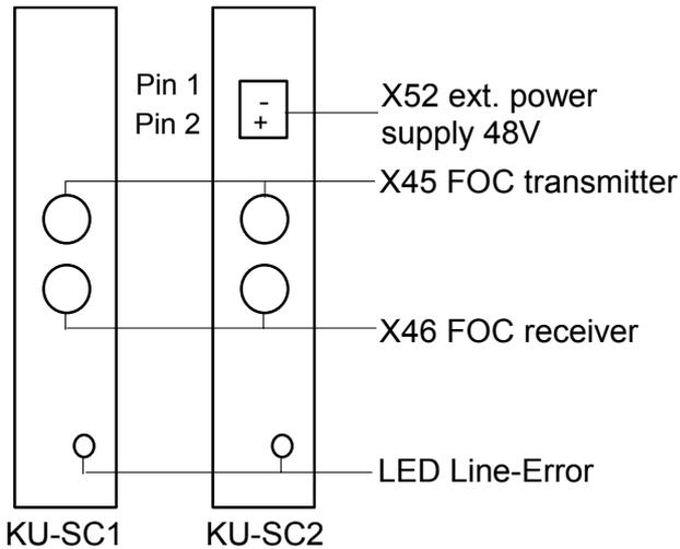
Fig.: Front panel of the modules KU-SC1 and KU-SC2
