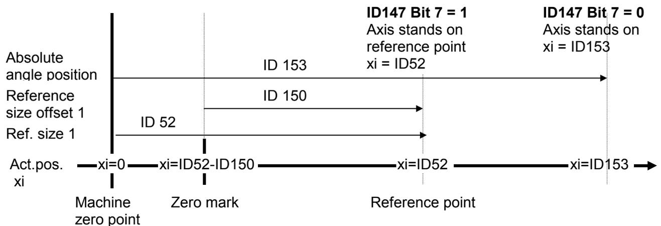
Figure: Effect of the parameters in the "Drive Controlled Homing Cycle" command
