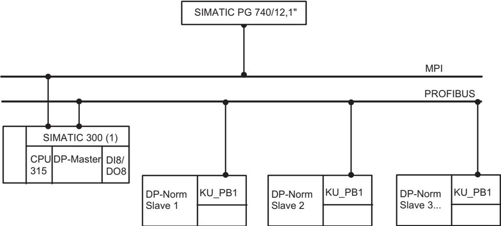
The driver software is multi axes capable: Several AMKASYN inverters (KW / KU) can be controlled by the AFP-S7-PB driver on the SIEMENS PLC.
