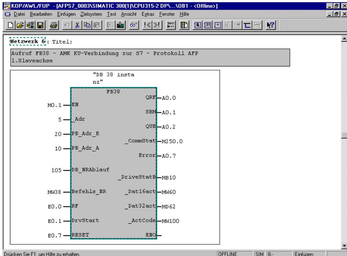
A DB38 instance is assigned to FB38. For each connected KU / KW inverter FB38 must be called-up anew. For each FB38 call-up an instance DB (DB38, DB39, ...) must be created and assigned to it.
