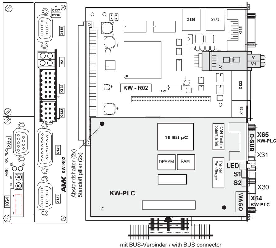
The KW-PLC can be used in slot 1 or 2.
