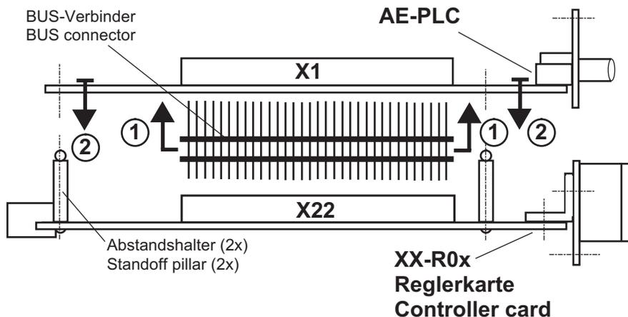
7. Push the controller card with the AE-PLC card as a whole carefully into the card shaft until the controller card is plugged securely in the mating connector.
