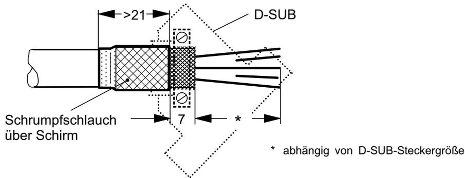
If shielded cables must be interrupted by connectors a continuous shield connection must be guaranteed by contacting the shield with all metallized connector housings. The shield may not be led via connector pins.
