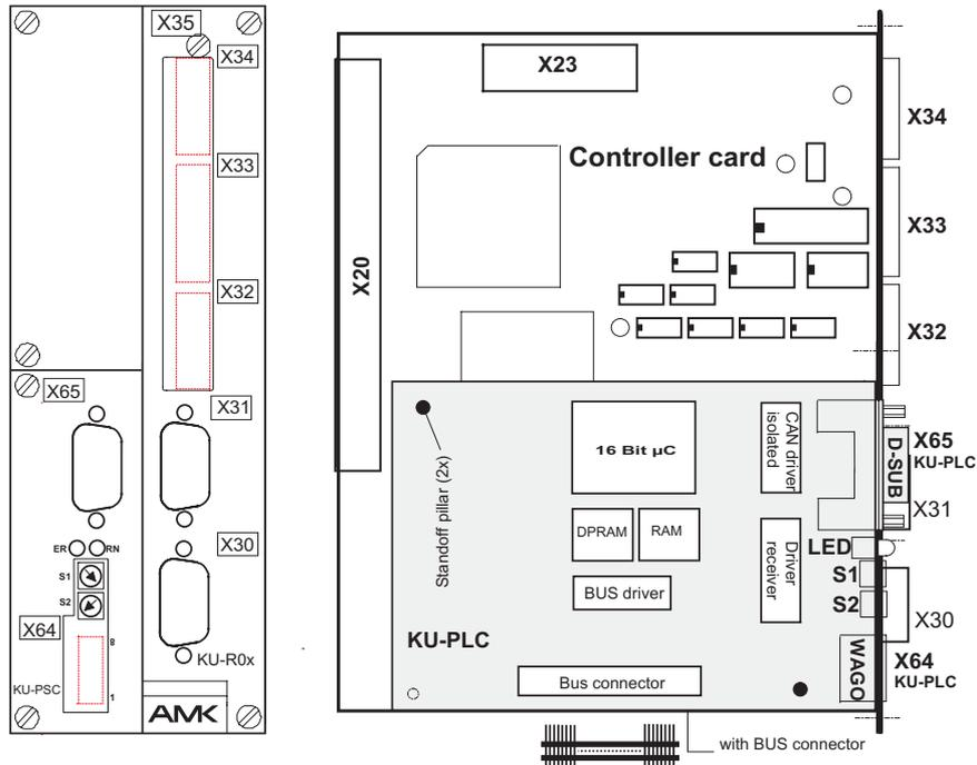
Figure 3-1 KW-PLC front plate and board structure
