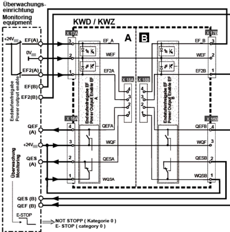
Power output enable single safety (A/B), one-channel (only EF):
