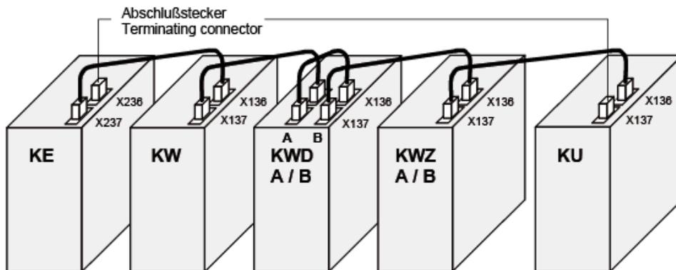
**Note:** Set a Bus terminating plug (120 Ohm) at the end and beginning of each line.
