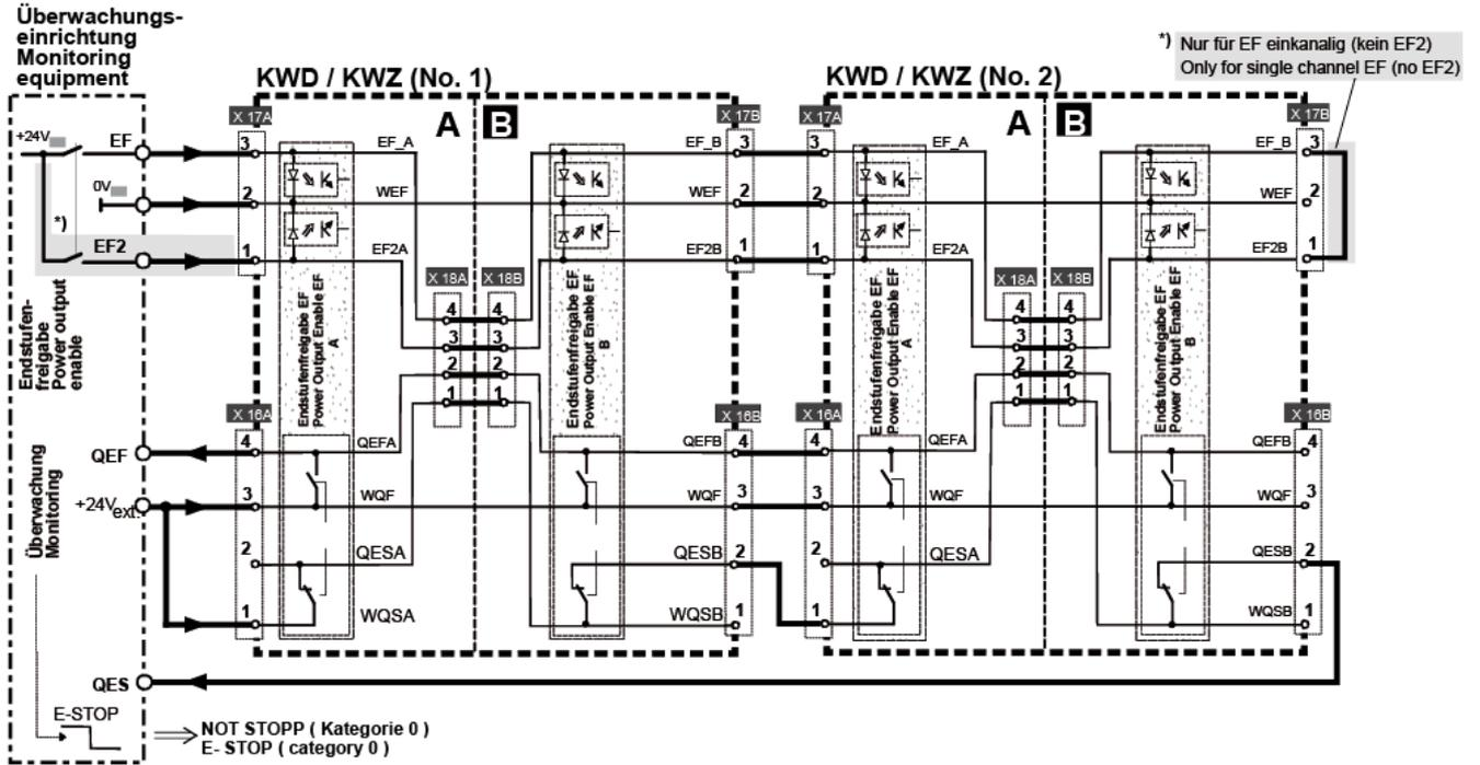
Power output enable single safety (A/B), two-channel (EF and EF2):
