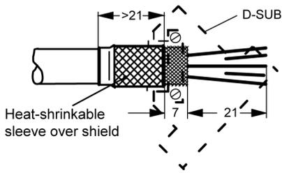
**Cable for signal plug connector**
