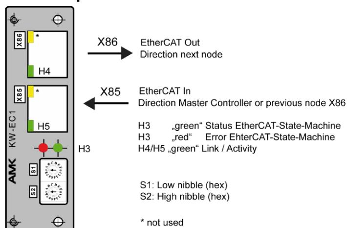
Picture name: ZCH\_KEKW\_KW-EC1\_Frontplatte
