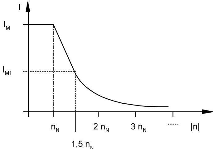
If ID32770 = ID32769 or ID32770 = 0 is set, the correction is eliminated and the magnetising current is proportionately reduced to  $1/n$  for speeds above the nominal speed.
