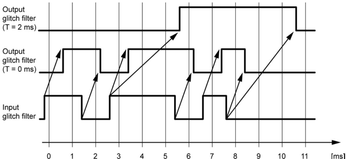
The glitch filter effects next behind the binary input for both directions. Positive and negative edge is not differentiated. For inputs parameterized as measuring inputs (probe function) the glitch filters have no function, no diagnosis message is generated.
