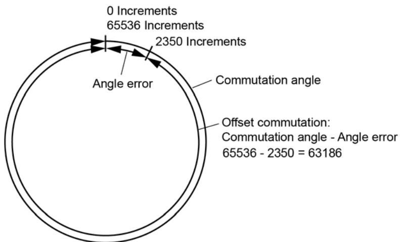
The electrically-aligned synchronous motor shows e.g. a commutation angle of ID32831 = 2350 increments (angle error). To compensate this value to 0, the commutation offset is calculated as follows:
