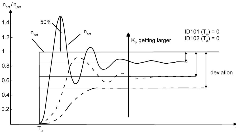
Course of the actual speed of the speed controller circuit for an erratic change of the speed setpoint depending on KP (ID100 ).
