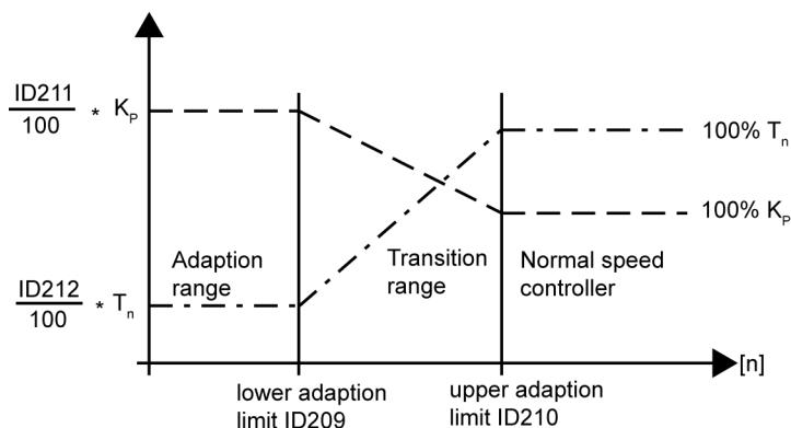
Below the lower adaptation limit,  $K_p$  and  $T_n$  work according to ID211 and ID212 and above the upper adaptation limit  $K_p$  and  $T_n$  work according to ID100 and ID101. Linear adaptation takes place in between.
