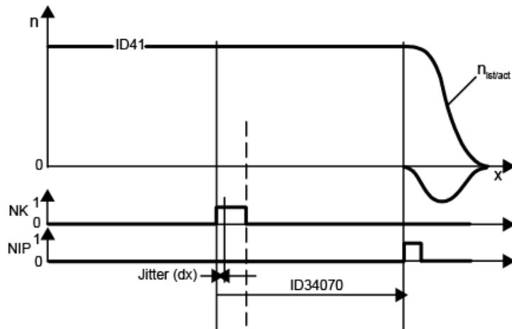
Due to the discrete sampling of the cam signal, a blur ( $dx$ ) results, whose size depends on the interpolator guide speed and the sampling time.
